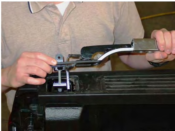
Roll rails to the outside of the pickup to remove
