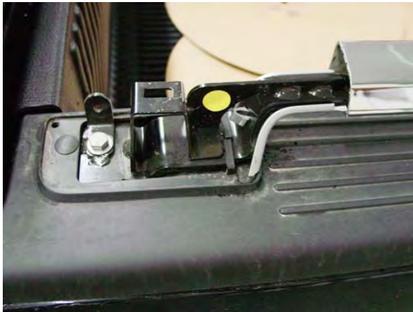
Start to loosen bolts at both ends of rails
