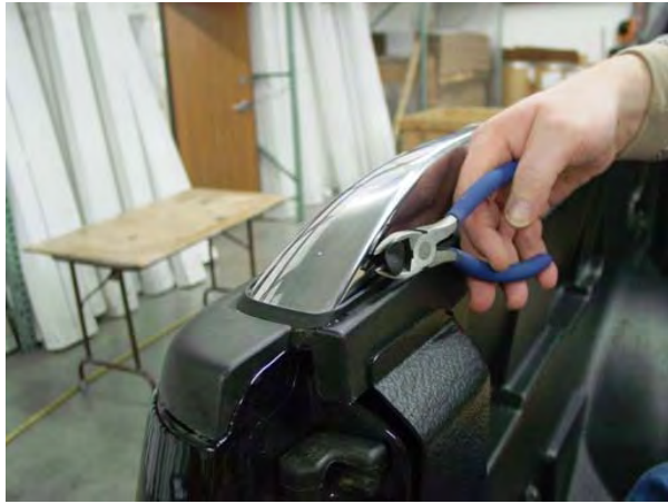
Remove black plastic clips on all 4 end caps
